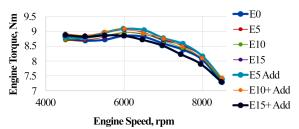
Fig. 5. Torque VS Engine Speed
