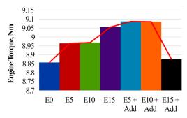
Fig. 6. Maximum Torques of 7 Fuel Variations
