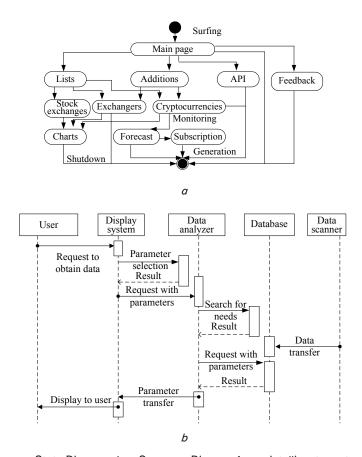
Fig. 3. Diagram: a- State Diagram; b- Sequence Diagram for an intelligent cryptocurrency system
