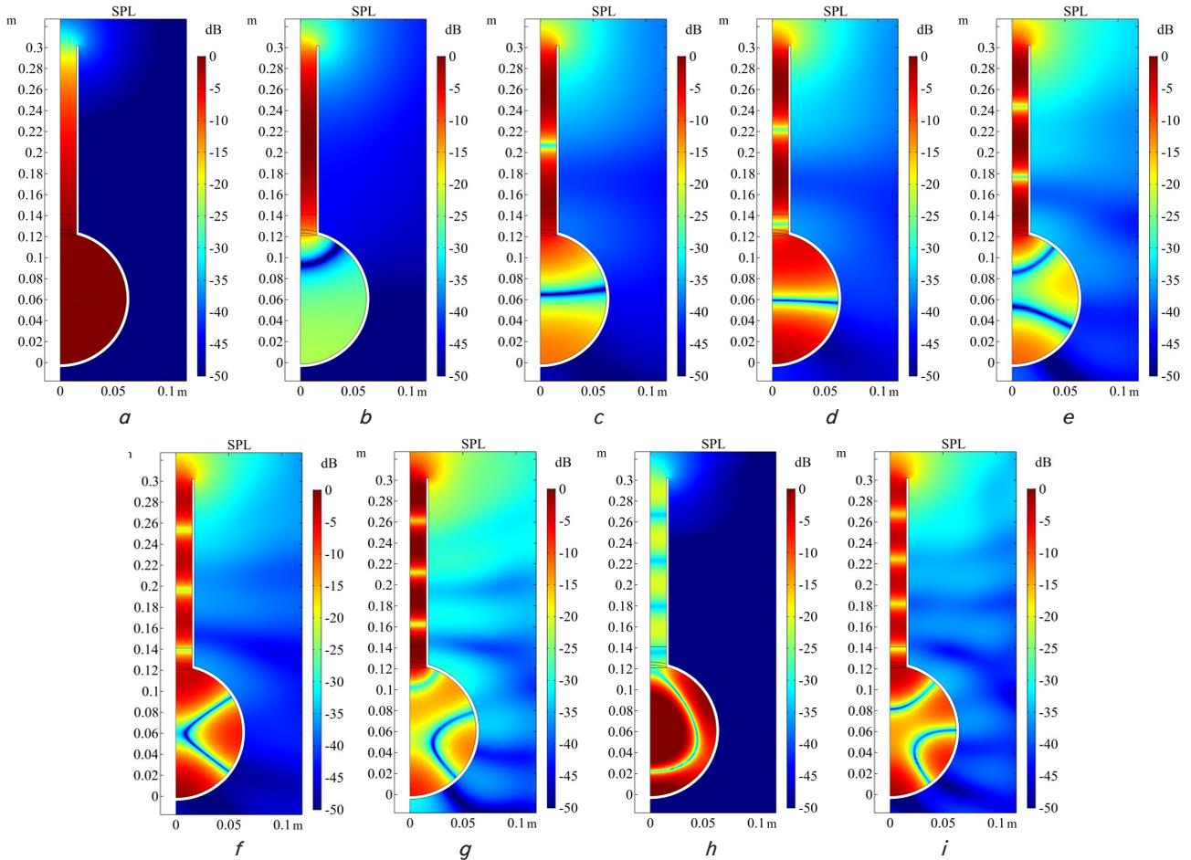
Fig. 3. Distribution of sound pressure levels in resonator No. 3 at the first nine resonance frequencies: *a* – 99 Hz; *b* – 892 Hz; *c* – 1,693 Hz; *d* – 1,947 Hz; *e* – 2,644 Hz; *f* – 3,038 Hz; *g* – 3,592 Hz; *h* – 3,962 Hz; *i* – 4,075 Hz
