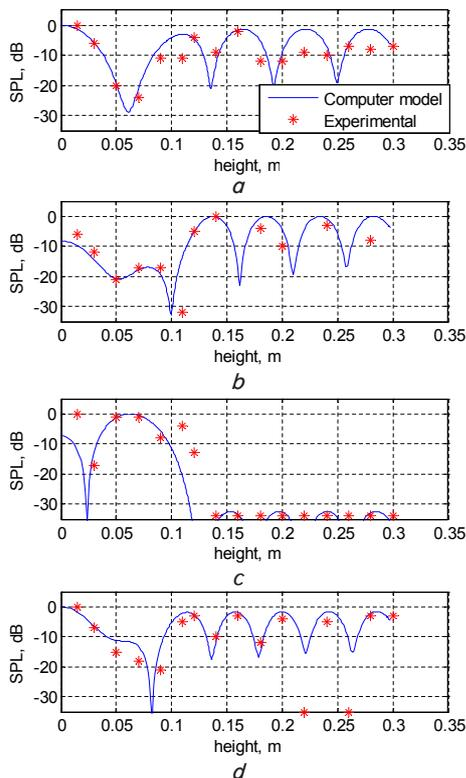
Fig. 5. Comparison of simulation results and experimental data for resonator No. 3, the sixth-ninth harmonic (the frequency of computer simulation is shown in brackets): a – 3,037 (3,038) Hz; b – 3,568 (3,592) Hz; c – 3,978 (3,962) Hz; d – 4,060 (4,075) Hz
