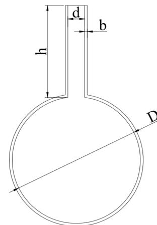
Fig. 1. General view of resonator
