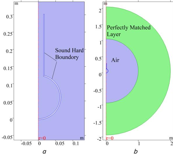
Fig. 2. Geometry of the resonator computer model: *a* – general view of the model; *b* – central part of the model (resonator)
