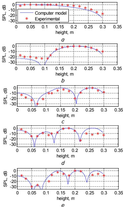
Fig. 4. Comparison of simulation results and experimental data for resonator No. 3, the first five harmonics (the frequency of computer simulation is shown in brackets): a – 99 (99) Hz; b – 893 (892) Hz; c – 1,681 (1,693) Hz; d – 1,947 (1,947) Hz; e – 2,625 (2,644) Hz
