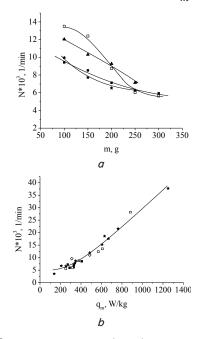
Fig. 3. Dependence of the grain drying rate on variable parameters: *a* - effect of mass, *b* - effect of the useful heat flow. ■ - wheat, □ - oats, ▲ - barley, ★ - buckwheat. The output power of the magnetron *P*=180 W
