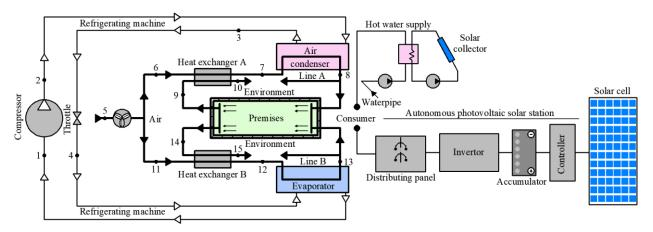
Fig. 4. Generalized technological scheme of a small trigeneration system
