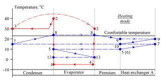
Fig. 6. Energy flows in the system "premises — refrigerating machine" in the heating mode
