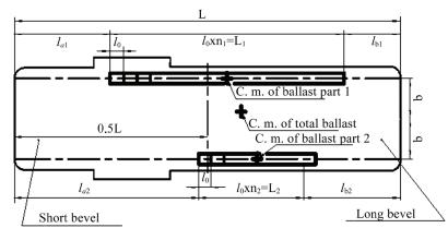
Fig. 2. Schematic of ballast arrangement
