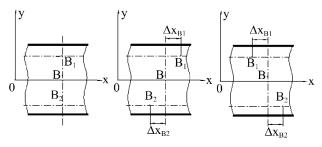
Fig. 4. Position of the centers of masses of ballast's parts
