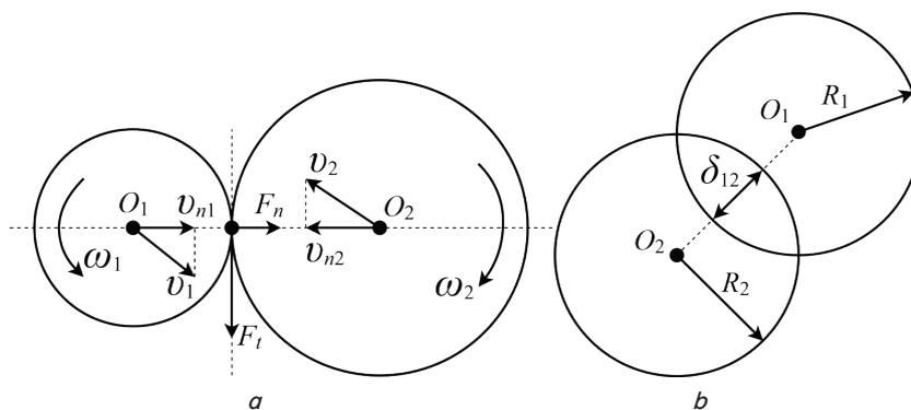
Fig. 2. Estimation schemes for determining parameters of particle interactions: a – forces of repulsion and friction; b – magnitude of the normal component of the force
