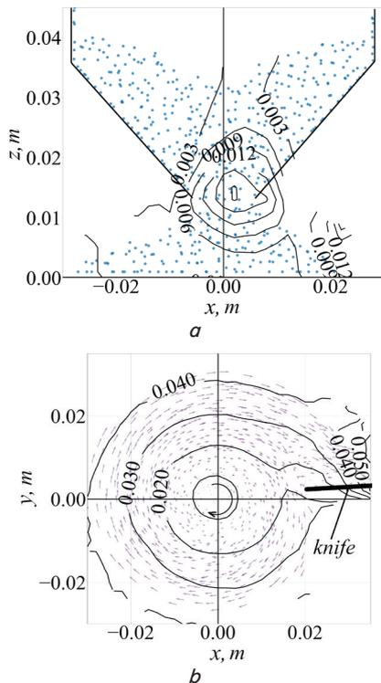
Fig. 4. Position, direction, and motion speed of particles: a – in the cross section of the system «hopper – feeder»; b – at the surface of the feeder's plate (top view)
