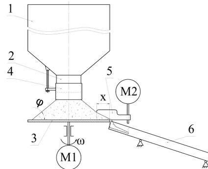
Fig. 1. System hopper – feeder
