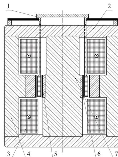
Fig. 10. Diagram of reciprocating motion electrodynamic linear motor: 1 – moving coil; 2 – magnetic flange; 3 – bias coil; 4 – magnetic housing; 5 – control coil; 6 – screen; 7 – rod
