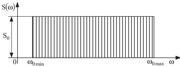
Fig. 3. Energy-efficiency optimal amplitude spectrum  $S(\omega)$
