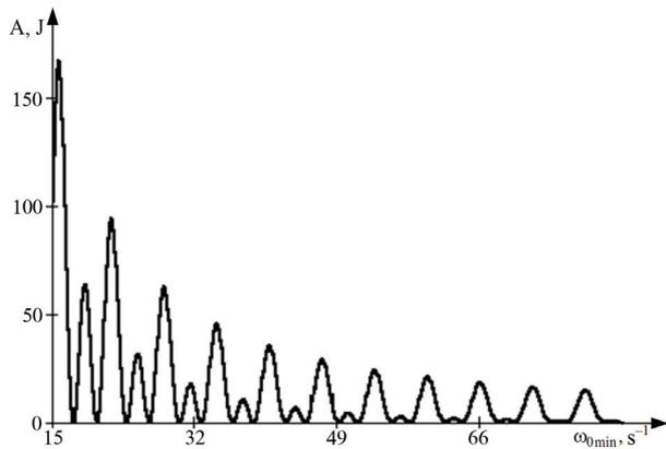
Fig. 8. Work dependency on  $\omega_{0min}$  for  $\omega_{0max} = 100 \text{ s}^{-1}$ ,  $S(\omega) = 4,000 \text{ N}$ ,  $m = 10 \text{ kg}$ , pulse duration – 1 s ( $\omega_{0min}$  is changed from 15 to  $100 \text{ s}^{-1}$ )
