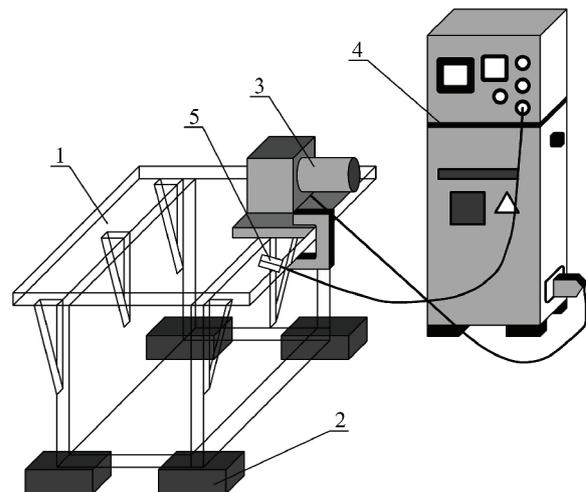
Fig. 2. Typical electromechanical vibration system with unbalanced mass: 1 – part; 2 – platform or vibration-insulating supports; 3 – vibration exciter; 4 – control panel; 5 – vibration sensor
