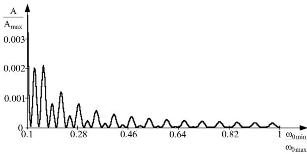
Fig. 9. Work dependency on  $\omega_{0min}$ , in relative units, pulse duration – 1 s
