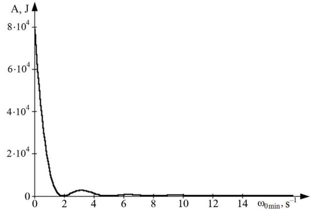
Fig. 7. Work dependency on  $\omega_{0\min}$  for  $\omega_{0\max}=100 \text{ s}^{-1}$ ,  $S(\omega)=4,000 \text{ N}$ ,  $m=10 \text{ kg}$ , pulse duration – 1 s ( $\omega_{0\min}$  is changed from 0 to  $15 \text{ s}^{-1}$ )
