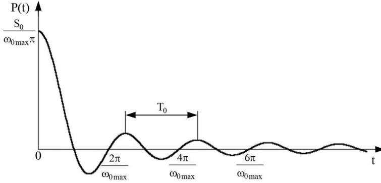
Fig. 6.  $P(t)$  plot, having an optimal spectrum for  $\omega_{0\min}=0$ , represented in the general form
