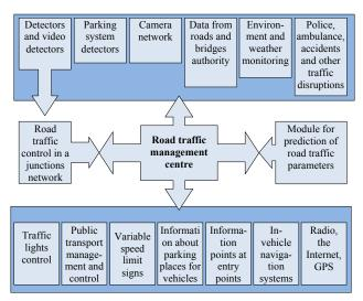
Fig. 7. Diagram of a road traffic management system
