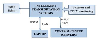
Fig. 2. An example of using intelligent transportation systems to manage road traffic
