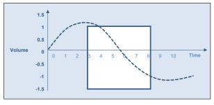
Fig. 8. Time window - input of neural network
