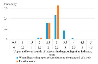
Fig. 3. Distribution density of the probability of intervals in the departure of transfer trains when they are organized at accumulation to the standard of a train
