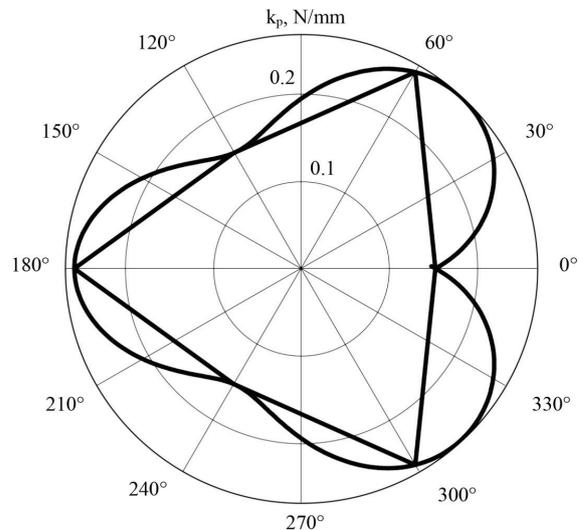
Fig. 7. Polar diagram of collet hardness in the polar system of polynomial approximation
