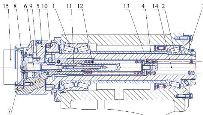
Fig. 1. Design scheme of the spindle unit with a clamping collet
