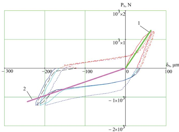
Fig. 5. Deformation of the cartridge-part system: 1 – when loading on the cam, 2 – when loading between the cams
