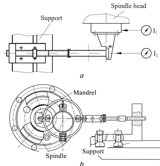
Fig. 4. Loading and measurement scheme: *a* – a view of the working area in the plan, *b* – a side view
