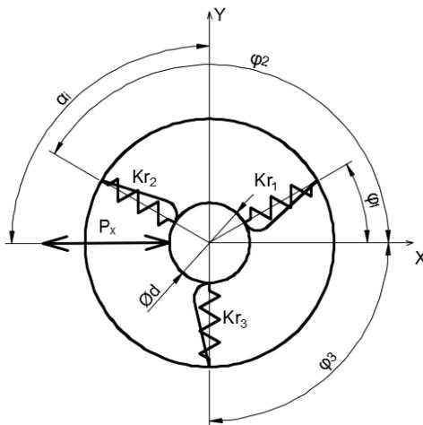
Fig. 6. Spatial position of the clamping elements and the load scheme
