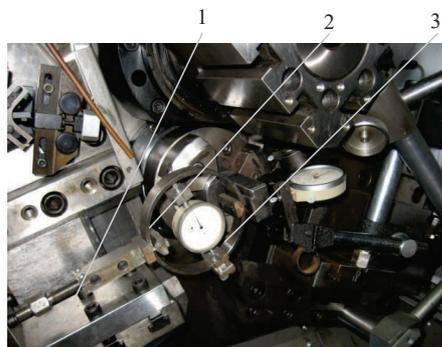
Fig. 2. Arrangement of equipment (the fitting) in the working area of the machine tool
