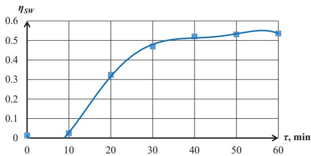
Fig. 9. A change in efficiency  $\eta_{\text{sw}}$  of the solar window throughout the experiment under the mode of gravitation motion of the heat carrier at radiation of solar energy simulator onto the setup at intensity  $600 \text{ W/m}^2$
