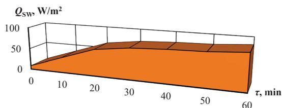
Fig. 11. Instantaneous power of solar window as solar collector  $Q_{\text{sw}}, \text{W/m}^2$  under the mode of gravity motion of heat carrier at the radiation of solar energy simulator onto the setup with intensity  $900 \text{ W/m}^2$
