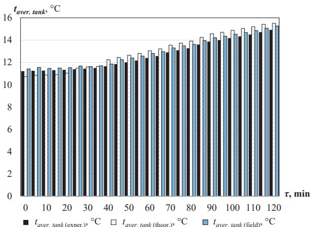
Fig. 10. Comparison of theoretical, experimental, and field data on temperature in the tank-accumulator of the solar window under the mode of gravity motion of heat carrier at radiation intensity  $900 \text{ W/m}^2$
