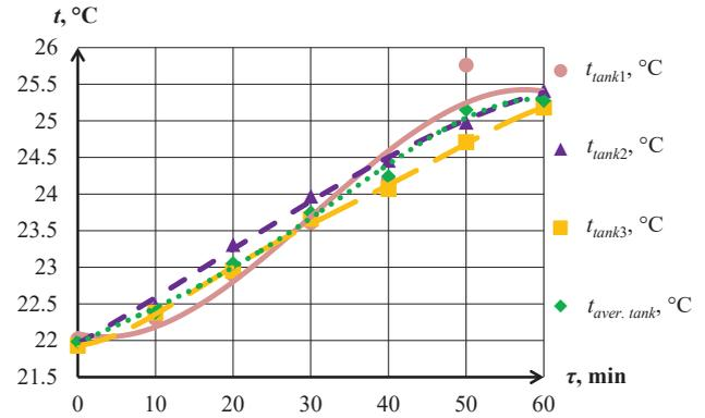
Fig. 6. A change of the temperature of the heat carrier in three layers of tank-accumulator  $t_{tank1...3}$ , °C and averaged temperature of the tank-accumulator  $t_{aver.tank}$ , °C depending on heating duration under the mode of motion of heat carrier circulation at radiation of the solar energy simulator onto the setup at intensity of 600 W/m<sup>2</sup>
