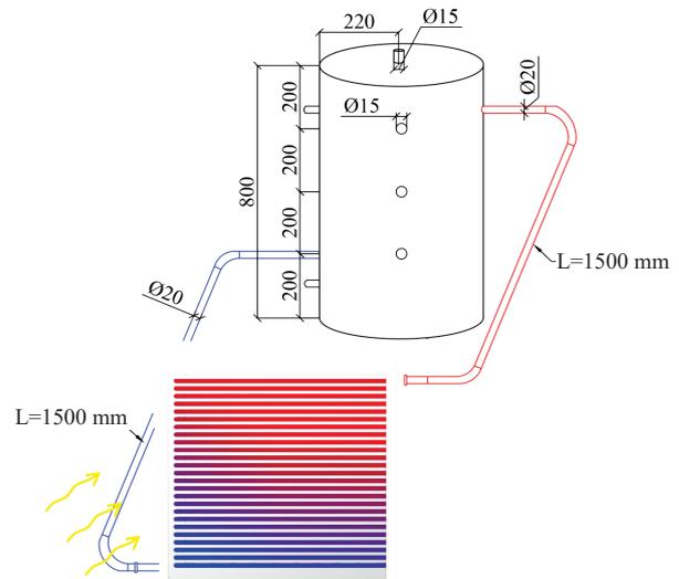
Fig. 4. Schematic of experimental setup of the system of solar heat supply with a solar window
