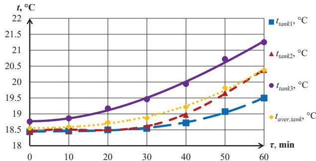
Fig. 8. A change in the heat carrier temperature in three layers of tank-accumulator  $t_{\text{tank}1...3}, ^\circ\text{C}$  and the averaged temperature of tank-accumulator  $t_{\text{aver.tank}}, ^\circ\text{C}$  depending on the duration of heating under the mode of gravitation motion of heat carrier at the radiation of solar energy simulator onto the setup with intensity  $600 \text{ W/m}^2$
