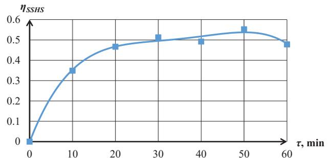
Fig. 7. Dynamics of change in efficiency of the system of solar heat supply with the solar window  $\eta_{SSHS}$  in general (at accumulation of thermal energy in the tank-accumulator) depending on duration of heating under the mode of heat carrier circulation motion at the radiation of the solar energy simulator onto the setup at the intensity of 600 W/m<sup>2</sup>
