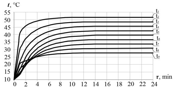
Fig. 3. Distribution of temperatures in the nine-section tank-accumulator over 24 hours
