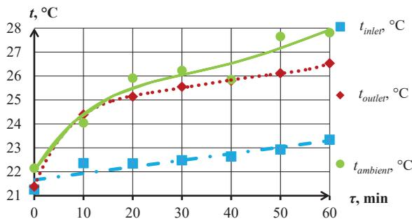
Fig. 5. Temperature of the heat carrier at the inlet  $t_{inlet}$ , °C and at the outlet  $t_{outlet}$ , °C of the solar window and the ambient temperature  $t_{ambient}$ , °C throughout the experiment under the mode of heat carrier circulation under conditions of radiation of the solar energy simulator on the setup at the intensity of 600 W/m<sup>2</sup>
