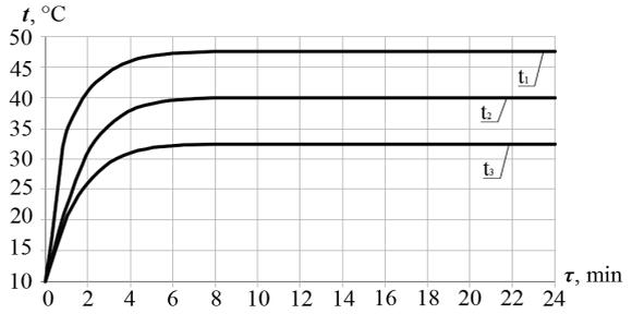
Fig. 2. Distribution of temperatures in the three-section tank-accumulator over 24 hours
