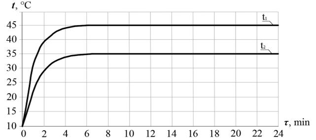
Fig. 1. Distribution of temperatures in the two-section tank-accumulator over 24 hours
