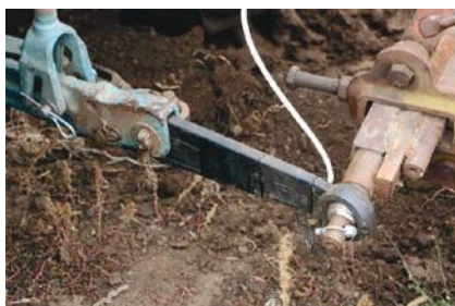
Fig. 10. The physical appearance of the strain gauge installed at the left link of the tractor’s attachment
