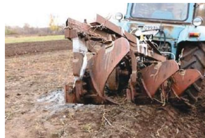
Fig. 13. The side view of a landside with the strain sensor mounted at the bearer of a third casing of the plough
