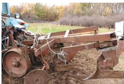
Fig. 15. The physical appearance of the tractor MTZ-82 with the mounted ploughshare PLN-3-35 and the landside with a strain sensor installed at the bearer of a second casing of the plough
