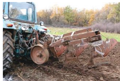
Fig. 12. The physical appearance of the tractor MTZ-82 with mounted ploughshare PLN-3-35 and a landside with the strain sensor mounted at the bearer of third casing of the plough
