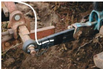
Fig. 9. The physical appearance of the strain gauge installed at the right link of the tractor’s attachment
