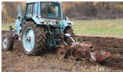
Fig. 8. Physical appearance of a machine-tractor assembly consisting of the tractor MTZ-82 and the mounted ploughshare PLN-3-35 with the installed measurement system and sensors
