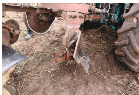
Fig. 17. The physical appearance of the tractor assembly with the mounted ploughshare PLN-3-35 and the landside with the strain sensor installed at the bearer of a first casing of the plough
