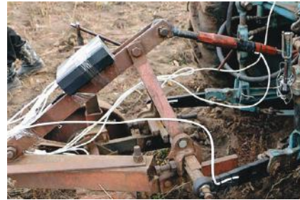
Fig. 11. The physical appearance of the strain gauge installed at the medium link of the tractor’s attachment
