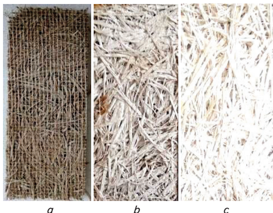
Fig. 1. Model samples of heat- and soundproofing material: a – based on wood wool – inorganic binder at the ratio of 1:1, b – based on wood wool – inorganic binder at the ratio of 1:2, c – based on wood wool – organic-mineral binder at the ratio of 1:1
