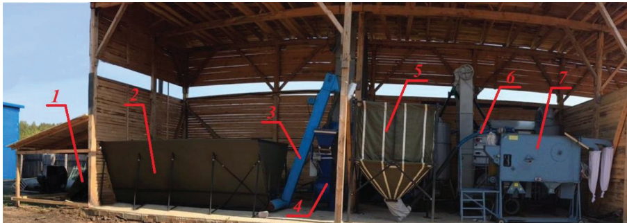
Fig. 6. A device for accepting and drying high-moisture soya piles under production conditions (air-slide conveyor): fan (1), cloth air-slide conveyor (2); scraper conveyor (3); pneumatic separator (4); storage bin (5); conveyor (6); fractional pneumatic separator (7)
