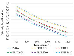
Fig. 1. Dependence of viscosity of melts of glass frits on temperature
