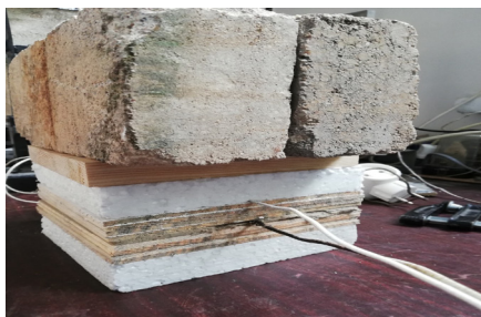
Fig. 4. Process of determining the thermal conductivity of the wood sample under the action of the heater
