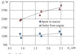
Fig. 8. Thermal power of exhaust gases
