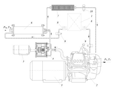
Fig. 1. Principal diagram of the energy-generating unit with a deep recovery of heat from exhaust gases: 1 - discharge tank with liquid fuel; 2 - internal combustion engine 1Ch 6.8/5.4; 3 - generator of electric current; 4 - rotary-piston expansion machine; 5 - generator of low power electric current; 6 - reactor for fuel conversion; 7 - synthesis gas cooler;
