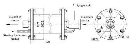
Fig. 3. Reactor for fuel conversion
