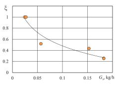
Fig. 7. Dependence of conversion degree on the mass flow rate of ethanol through the reactor
