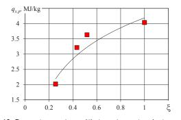
Fig. 10. Dependence of specific heat from chemical reaction on conversion degree
