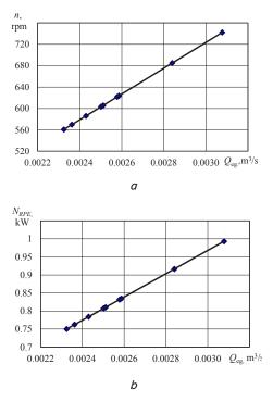
Fig. 4. Dependences of parameters for a rotary-piston engine on the flow rate of a working body: a – rotor rotation frequency; b – effective power
