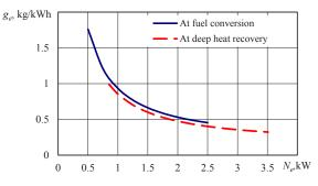
Fig. 11. Dependence of specific effective fuel consumption on effective power of the energy-generating unit
