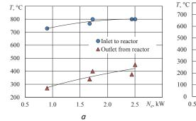
of synthesis gas at the outlet from the reactor) (Fig. 6) at approximation accuracy  $R^2$ =0.96, as well as the dependence of conversion degree on the mass flow rate of ethanol through the reactor (Fig. 7) at approximation accuracy  $R^2$ =0.93.
