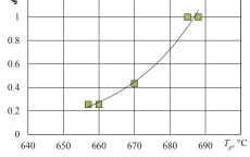
Fig. 6. Dependence of ethanol conversion degree on the reaction temperature
