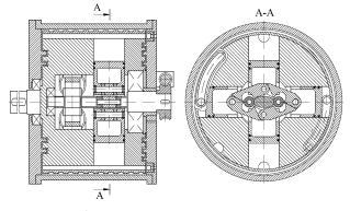
Fig. 2. A rotary-piston expansion machine
