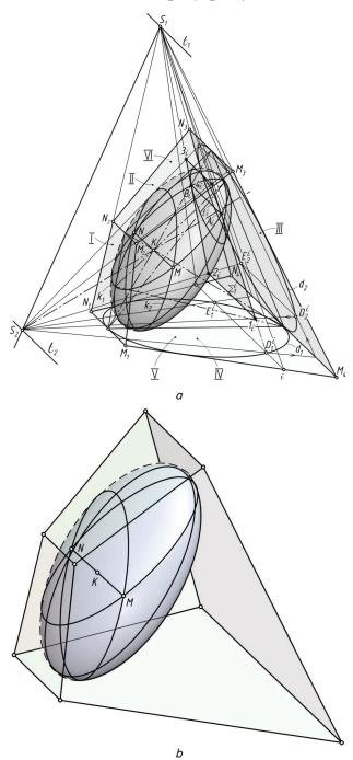
Fig. 5. A hexagon, which limits the quadric surface, assigned by two tangent cones: a — geometric scheme of construction of quadric; b — images of the quadric that is tangent to the hexagon faces
