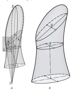
Fig. 6. Example of a change in the shape of conjugate quadrics: a — geometric scheme; b — example of the changed shape
