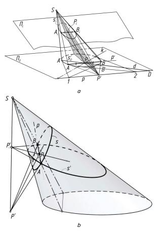
Fig. 1. Property about the centers of conic cross-sections in bundles of planes: a — axis of the bundle does not cross the cone; b — axis of the bundle crosses the cone
