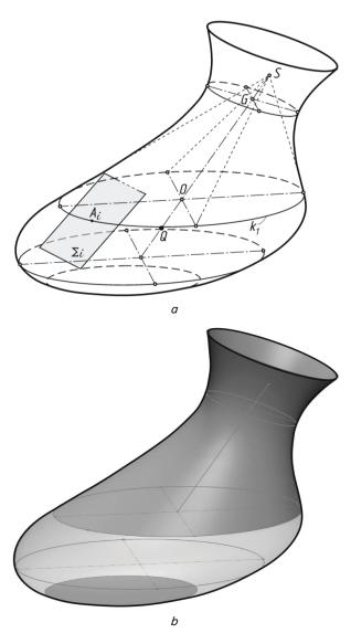
Fig. 8. The surface of the vase from conjugate quadrics: a – geometric scheme; b – appearance
