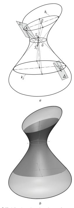
Fig. 7. Modeling the surfaces from three conjugate quadrics: a- geometric scheme; b- appearance
