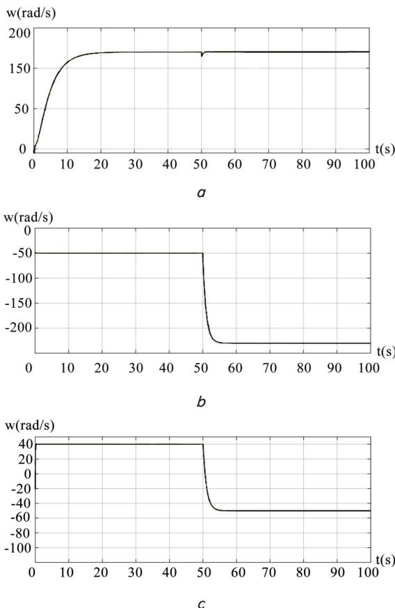
Fig. 5. Transient process of the combined invariant ACS of engine angular speed taking into account the influence of the compensating device: *a* – output characteristic of the ACS; *b* – characteristic of the initial value of the disturbance; *c* – output signal characteristic of the device limiting the maximum permissible value of disturbance
