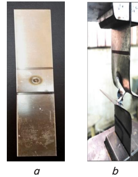
Fig. 6. Spot welded specimen: a – before the tensile test; b – after the tensile test
