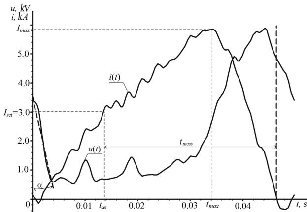
Fig. 8. Oscillograms of transitional electric magnitudes when disabling HSS VAB-206 at close SC,  $l=2\text{ km}$ ,  $I_y=3,000\text{ A}$
