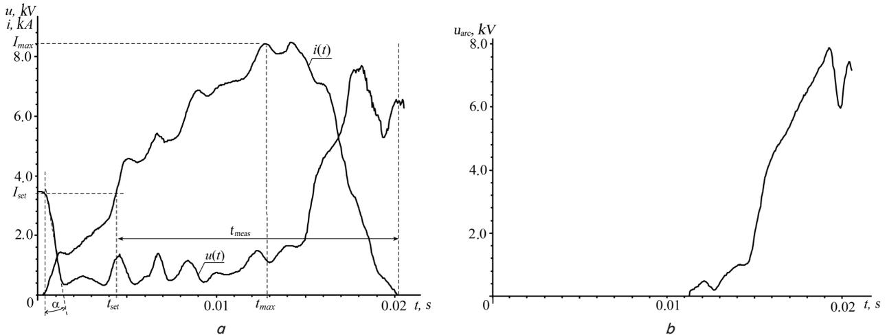
Fig. 5. Oscillograms of change in transitional electric magnitudes when disabling HSS 2×VAB-43 at close SC,  $l=0.5$  km, the setpoint current  $I_y=3,500$  A: *a* – time dependences of feeder current  $i(t)$  and voltage  $u(t)$ ; *b* – voltage on the electric arc of a high-speed circuit breaker  $u_{arc}(t)$
