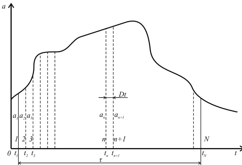
Fig. 2. Discretization of a continuous pulse of transition magnitude  $a(t)$
