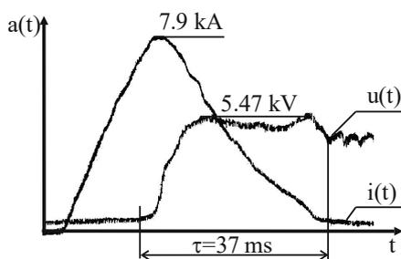
Fig. 1. Oscillographs of transitional feeder voltage  $u(t)$  and current  $i(t)$  when disabling a short circuit in a traction network with a high-speed switch the type of AB-2/4
