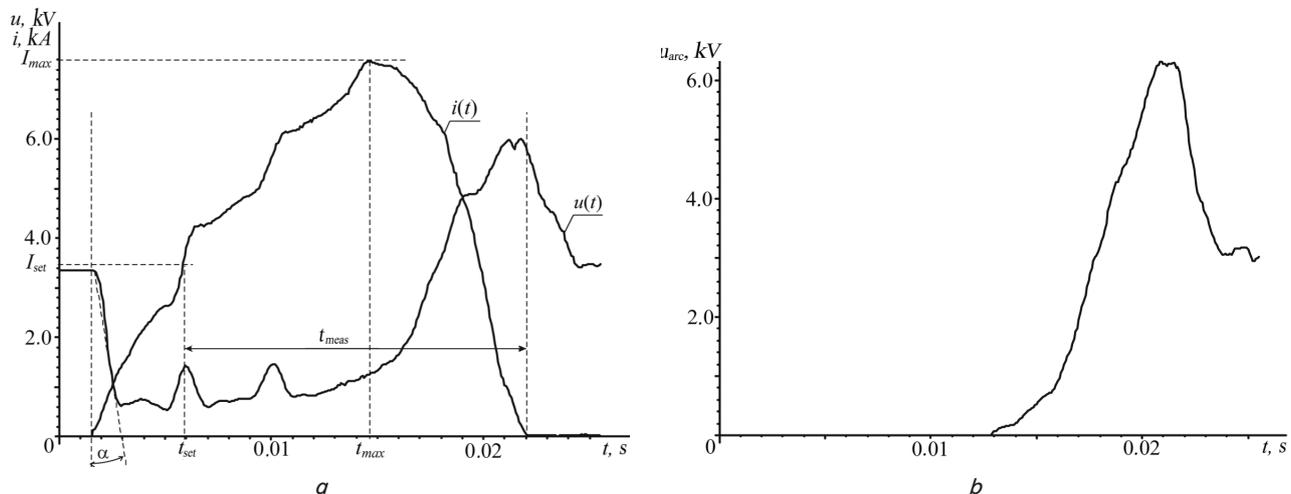
Fig. 6. Oscillograms of transitional electric magnitudes when disabling HSS 2×VAB-49 at close SC,  $l=0.5$  km,  $I_y=3,500$  A: *a* – time dependences of feeder current  $i(t)$  and voltage  $u(t)$ ; *b* – voltage on the electric arc of a high-speed circuit breaker  $u_{arc}(t)$
