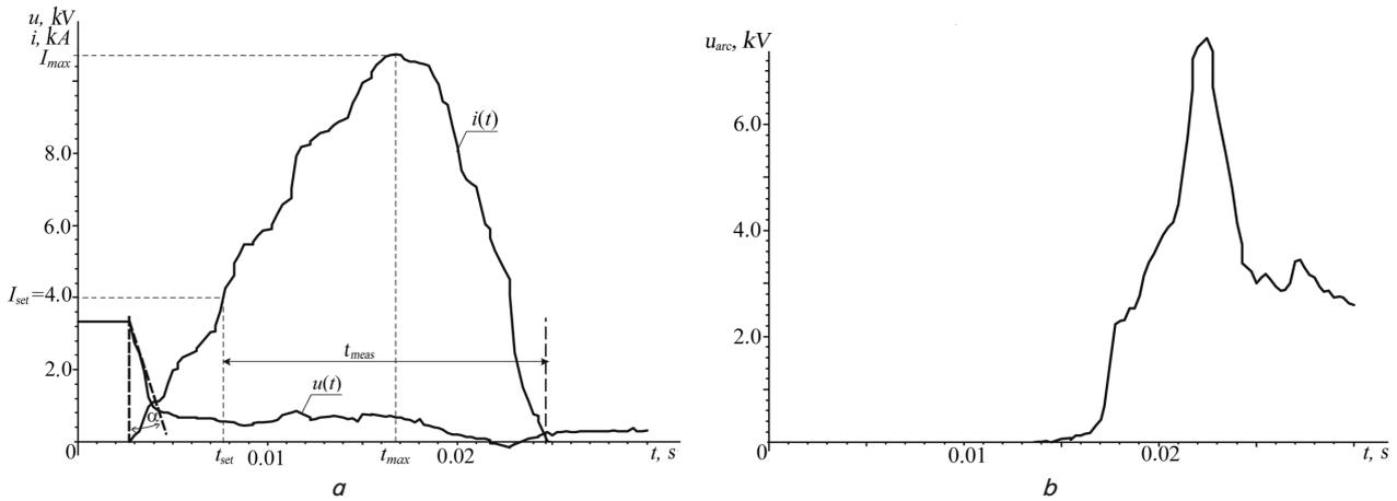
Fig. 7. Oscillograms of transitional electric magnitudes when disabling HSS VAB-206 at close SC,  $l=0.5\text{ km}$ ,  $I_y=4,000\text{ A}$ : a – time dependences of feeder current  $i(t)$  and voltage  $u(t)$ ; b – voltage on the electric arc of a high-speed circuit breaker  $u_{arc}(t)$
