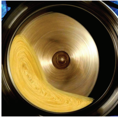
Fig. 2. A pattern of steady-state fill motion with relative particle size d/(2R)=0.01...0.03 at the chamber filling degree \kappa=0.25 ; the chamber rotates with relative velocity \psi_{\omega}=0.75
