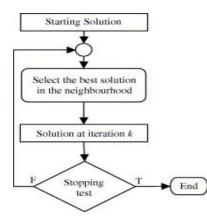
Figure 4 – Simple hill climbing algorithm flowchart
