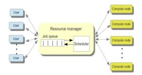
Figure 1 – Resource manager and communication between users and nodes
