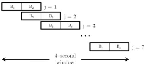
Figure 4 - Structure of the sliding window. In this figure,  $j$  represents a counter which is incremented each time a new data block arrives. As indicated earlier,  $B_j$  refers to a block of data which contains 125 data samples (approximately 0.5 seconds).
