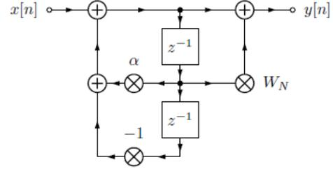
Figure 3 – Block diagram of the used Goertzel algorithm
