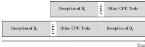
Figure 5 - Task scheduling. The DMA controller let the processor perform other operations while the data were being received. The block notation refers to the one used in the Figure 4.
