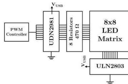
Figure 2 –The schematic diagram of the LED matrix driver. The UDN2981 was set to source roughly 350 mA and the ULN2803 was able to sink the same amount of current.
