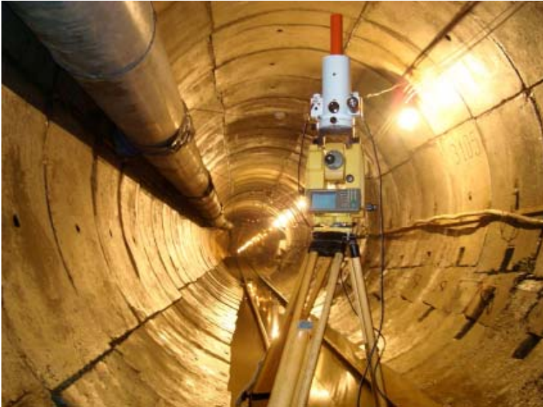
Pict. 2. GYROMAX AK-2M on the basis of total station GTS-722 to 100 mm) by building underground and hydrotechnic tunnels permitted rates. GMT Heger and UKRKOVID NVP GROUP companies make plans about implementation of GYROMAX AK-2M gyroscopic adapter in Russia.
