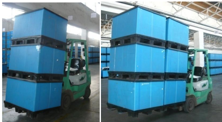
Fig. 4. The use of traditional and extended forks in the store of BJE Conclusion.
