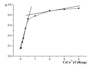
Fig. 4. Dependence of toluene extract optical density from the ratio of components in the system  $\text{Co}^{2+} - 1$ -(5-benzyl-2-thiazolyl)-azo-2-naphthol;  $C(\text{Reag}) = 5.8 \cdot 10^{-5} \text{ M}, \text{ pH} = 12, 1 = 1,0 \text{ cm}, \lambda = 565 \text{ nm}$
