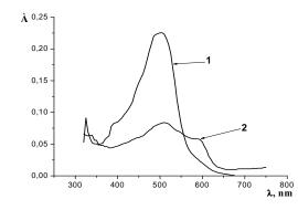
Fig. 6. The absorption spectrum of 1-(5-benzyl-2-thiazolyl)-azo-2-naphthol in toluene solution in the absence (1) and in the presence (2) of Ni<sup>2+</sup> ions;  $C(\text{Reag}) = 1.5 \cdot 10^{-5} \text{ M}, C(\text{Ni}^{2+}) = 7.5 \cdot 10^{-5} \text{ M}, C(\text{NaOH}) = 8.0 \cdot 10^{-2} \text{ M}, 1 = 1.0 \text{ cm}$
