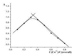
Fig. 5. Setting the ratio of the interaction in the system Co(II) – 1-(5-benzyl-2-thiazolyl)-azo-2-naphthol by the method of continuous variations;  $C(total) = 9.0 \cdot 10^{-5} \text{ M}, \text{ pH} = 12, 1 = 1,0 \text{ cm}, \lambda = 565 \text{ nm}$
