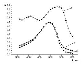
Fig. 7. The absorption spectrum of 1-(5-benzyl-2-thiazolyl)-azo-2-naphthol in toluene solution at the presence of Ni<sup>2+</sup> ions in the initial solution after preliminary separation of nickel by triple extraction of its dymethylglyoksimate into chloroform,  $C(Reag) = 4,5 \cdot 10^{-5} \text{ M}$ , m(Ni) = 2.2 mg (1); 0.44 mg (2); 0.22 mg (3);  $C(NaOH) = 8.0 \cdot 10^{-2} \text{ M}$ , l = 1.0 cm.
