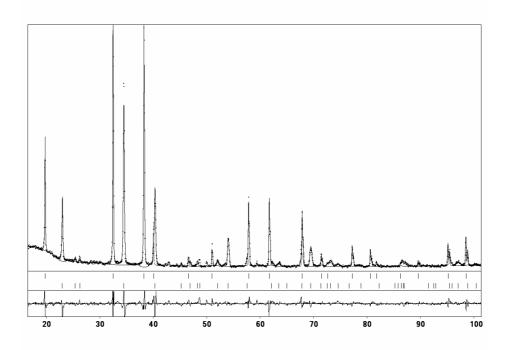
Figure 3. Experimental, calculated and difference diffraction patterns of the two-phase sample with composition  $Ho_{33}Zn_{20}Al_{47}$  (Cu-K $\alpha$  radiation)
