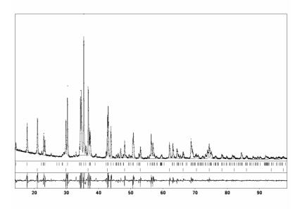
Figure 2. Experimental, calculated and difference diffraction patterns of the two-phase sample with the composition  $Ho_{21}Zn_{25}Al_{54}$  (CuK $\alpha$  radiation)
