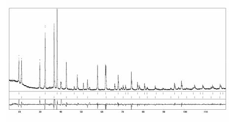
Figure 1. Experimental, calculated and difference diffraction patterns of the two-phase sample with the composition  $Ho_{25}Zn_{17}Al_{58}$  (CuK $\alpha$  radiation)
