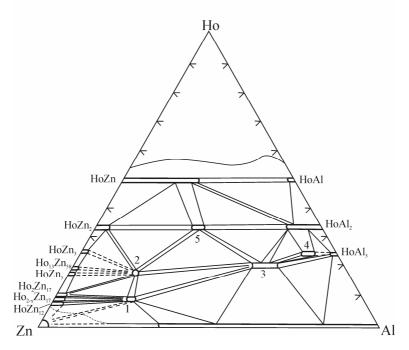
Figure 4. Phase diagram of the Ho–Zn–Al system at 500°C and 0–50 at. % Ho
