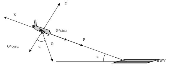
Fig. 1. Aircraft forces chart at glide slope (RWY is runway)
