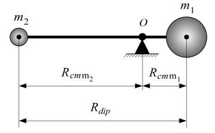
Fig. 5. The kinematic scheme of the virtual meter of "dipole" type at experiment 2
