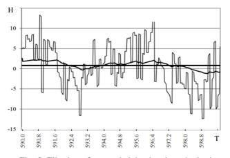
Fig. 8. Filtering of sensor height signal on the basis of discrete optimal fuzzy filter with a nonstationary wind disturbance
