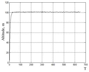
Fig. 6. Measurement of the UAV height signal using Kalman-Bucy filter with a known stationary noise
