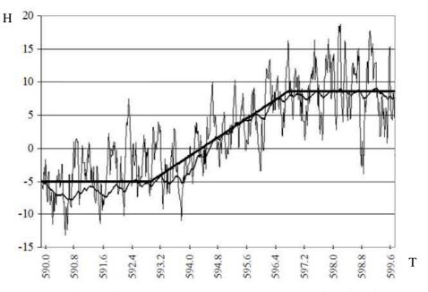
Fig. 4. True, noisy and filtered signal, at the optimum parameters of the filter function
