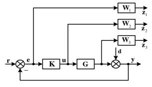
Fig. 3. The structural chart for the method of mixed sensitivity
