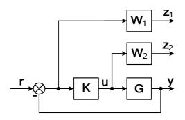
Fig. 2. The structural chart of the control system with the weigh transfer functions
