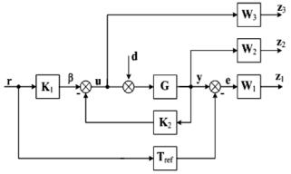
Fig. 4. The problem statement of the 2DOF controller synthesis by the method of mixed sensitivity
