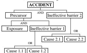
Fig. 4. Schematic fault tree structure
