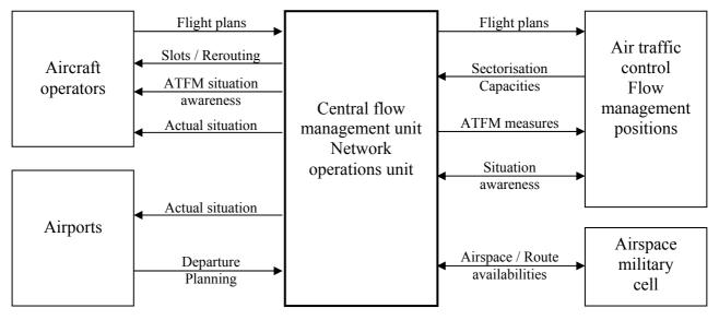
Fig. 2. Operational Structure with CFMU Network Operations Unit
