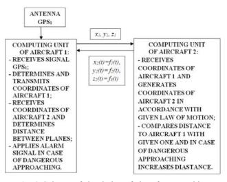
Fig. 4. Scheme of simulation of aircraft approaching
