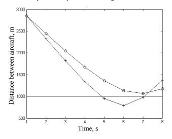
**Fig. 5.** Dependence of the distance between the aircraft on time: curve, marked by circles corresponds to the speed of approaching 412 m/s (1484 km/hour), and marked with crosses – 526 m/s (1893 km/hour)
