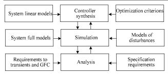
**Fig. 5.** Design of the robust regulator: GFC – gain-frequency characteristic
