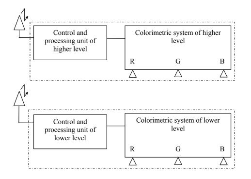
Fig. 1. Block-scheme of two-level RGB colorimetric system
