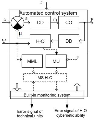
Fig. 6. ACS with the evaluation of EO state: MML – mathematical models of particular limit value  $\Psi$ ; MU – measure unit of  $\alpha_1$  parameters; MS H-O – measure system of H-O cybernetic ability
