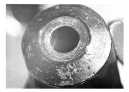
**Fig. 2.** Damage of the top end face surface of the slider (armature)
