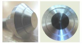
Fig. 10. Photos of the circular groove in the valve made of steel 08H18N10T after  $3 \cdot 10^5$  cycles
