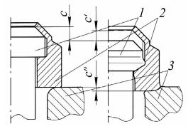
**Fig. 3.** Change in the relative position of locking washer (2), the head of the rod (1) and the slider (3).
