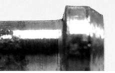
**Fig. 8.** Photos of valve drive rod head after resource loads: a - moving unit without damping device, operating time  $-20\ 000$  cycles; b - moving unit with the damping device, operating time  $-1\ 000\ 000$  cycles
