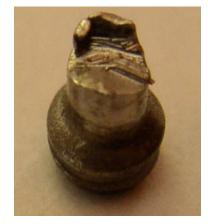
Fig. 6. Fatigue destruction of rod neck
