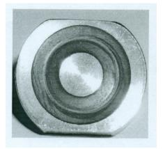
**Fig. 5.** Groove on the rubber surface of the rubber seal that is formed under the influence of operating loads
