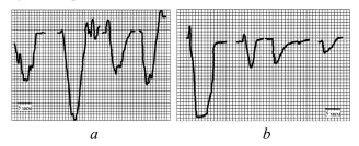
**Fig. 12.** Profile diagrams of the slide and saddle contacting areas after 300 000 cycles: a – without damping; b – with damping
