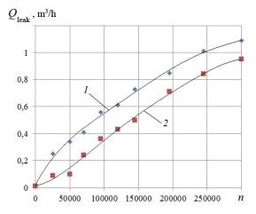
**Fig. 11.** Experimental dependencies of the leakage on the number of cycles:
