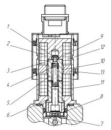
Fig. 1. Structural scheme of two-position valve with electromagnetic drive:
