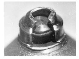
**Puc. 4.** Rod and slider mounting unite after valve lifetime end
