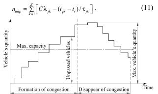
**Fig. 1.** Dynamics of formation and disappearance of queues of vehicles forming a queue of cars that has not passed through during one cycle of the traffic light
