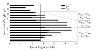
**Fig. 3**. Dynamics of the congestion queue formation at the intersection of the roadways
