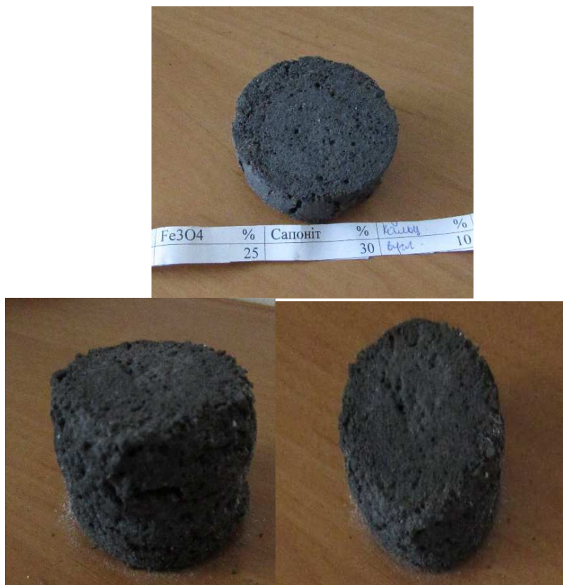
Fig. 2. New penetrating porous ceramics obtained by SHS
