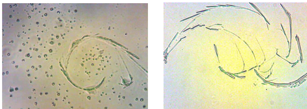
Fig.1 – Micrographs of fuel environment (MDO at the Left side with temperature 20° C, – marine heavy fuel oil IFO-360 at the right with temperature 52 °C)
