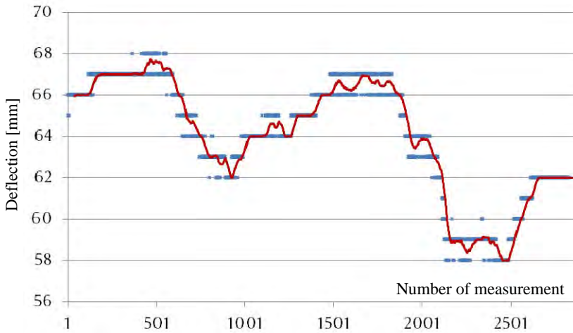
Fig. 21. Measured deflection of girder nr 47 on 5÷6 February 2012
