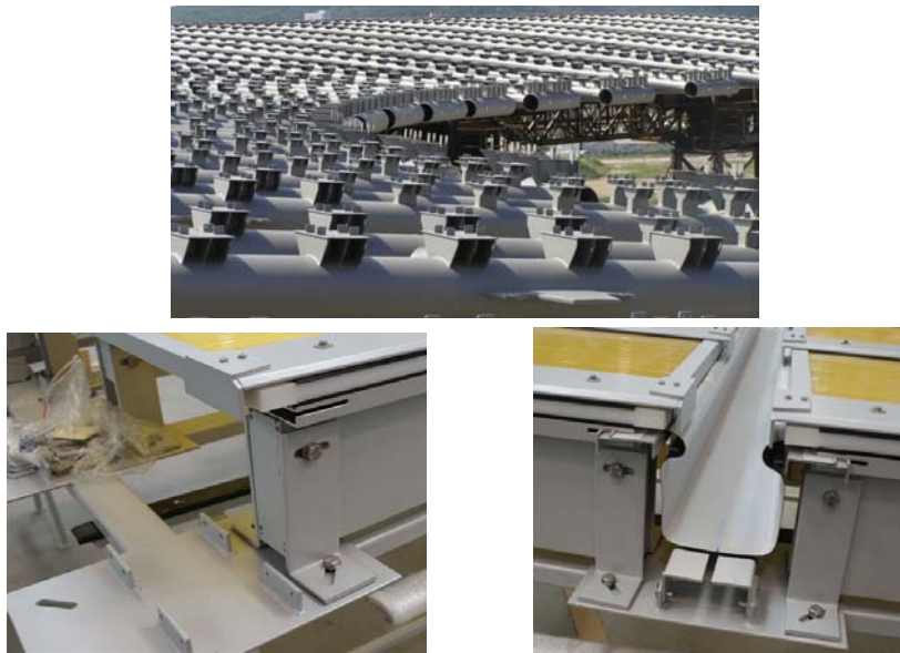
Fig. 6. The support structure of the covering
