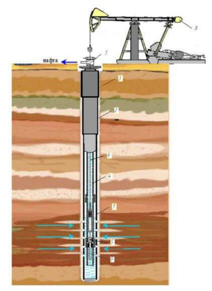
**Picture 2 – MAD operational procedure in the well:** 1 – capital string; 2 – intermediate string; 3 – surface casing; 4 – tubing; 5 – well pump; 6 – pump rod; 7 – tee; 8 – pumpjack; 9 – MAD
