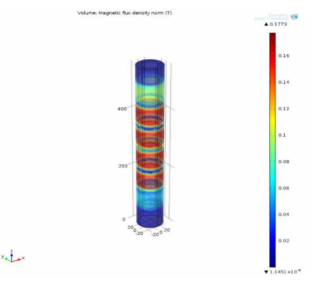
**Picture 10 – 3D model of magnetic induction distribution**
