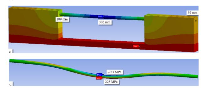
Picture 7 – Results of the hypothesis testing that pipeline deformation equivalent to soil deformations: a – uneven deformations for model with soil under pipe; b – longitudinal stresses for model with soil under pipe; c – pipeline deflection for model without soil; d – longitudinal stresses for model without soil
