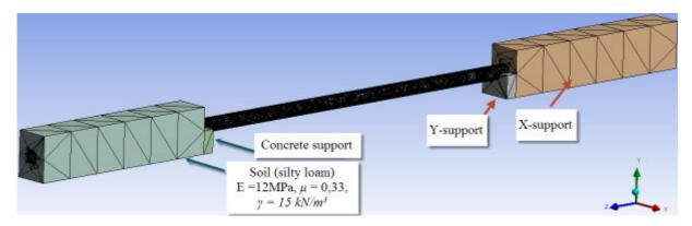
Picture 2 – Oil pipeline above ground crossing of the ravine design scheme
