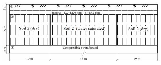
Picture 5 – Pipeline in the loessial soil with collapsible property (central area in the water saturated state, side areas in the natural condition)
