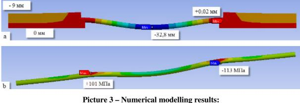
Picture 3 – Numerical modelling results: a – pipeline deflection; b – longitudinal stresses from deflection
