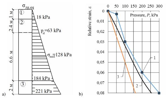
Picture 6 – Calculation of soil collapsible deformations from its own weight:
