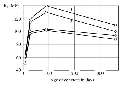
Figure 2 – Chart changing concrete strength (1), mortar (2) and cement (3) in time (based on the results of experiments V. Sytnyk, Yu. Ivanova)
