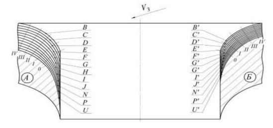
Figure 1 – Net depreciation experimental separating sieves after operating time: B - new; C - 100 t; D - 200 t; E - 300 t; F - 400 t; G - 500 t; H - 600 t; I - 700 t; J - 800 t; N - 900 t; P - 1000 t; U - 1080 t (wear limit); 0, I, II, III – line depreciation for the entire period of operating time;  $V_s$  – direction of the grain material.
