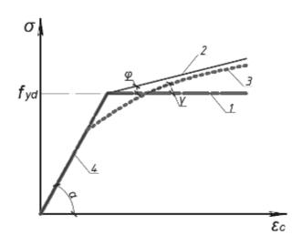
Figure 4 – Idealized steel deformation diagrams:
